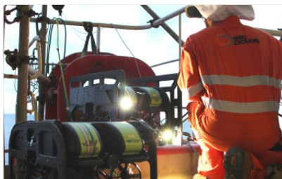
UNMANNED (ROV) HULL SURVEY PACKAGE
